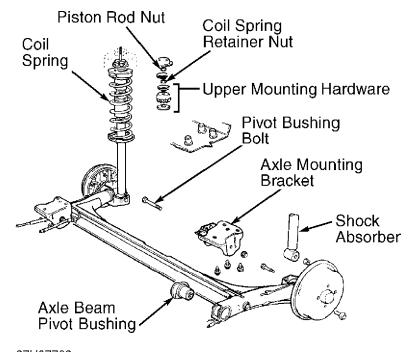
Fig. 1: Rear Suspension Assembly (Typical) Courtesy of Volkswagen United States, Inc.
