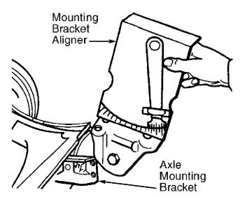
Fig. 2: Aligning Axle Beam Mounting Pad (Except Beetle)
